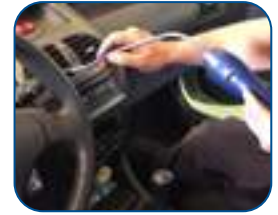
Leak in the evaporator.
